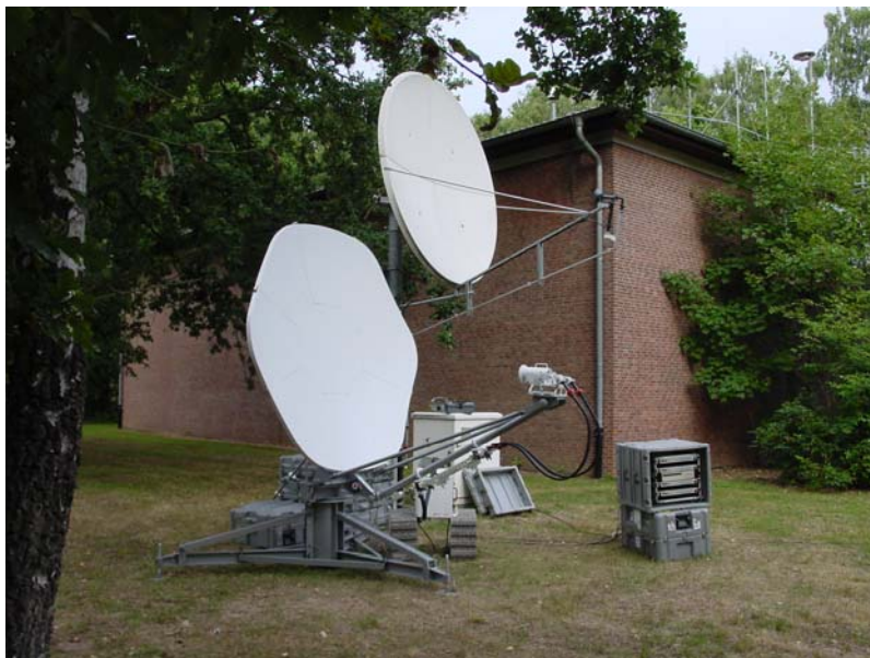
Figure 2. The Fly-away calibration apparatus (left) and the PTB operational station.
